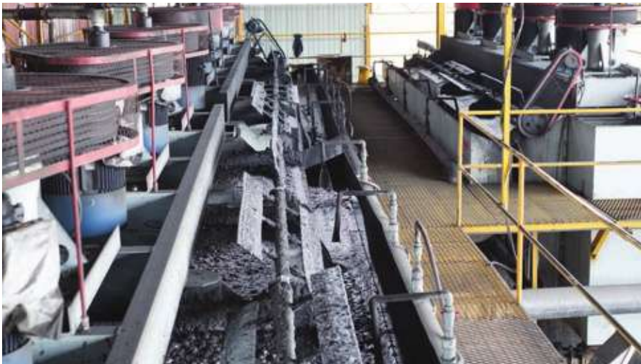
Diagram illustrating froth floatation cells
