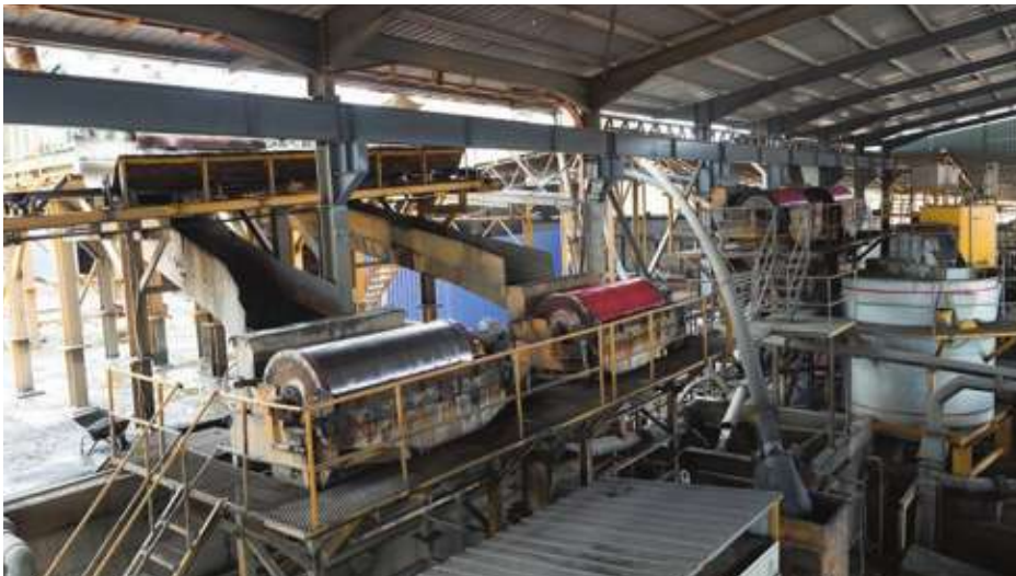
Diagram illustrating magnetic separator
