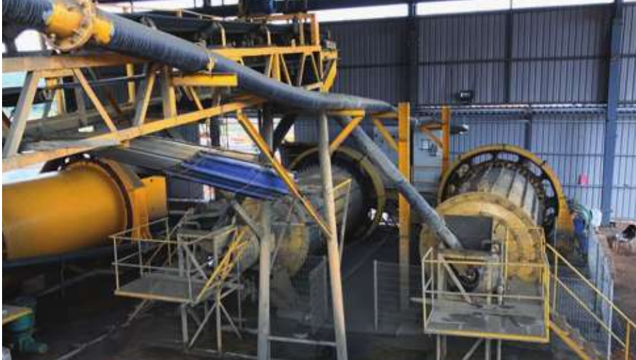
Diagram illustrating stage 1 grinding ball mills
