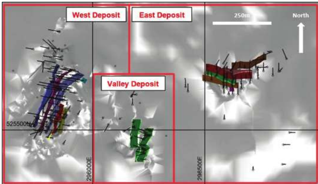
Figure 3-7: Drill collar locations and interpreted mineralisation wireframes
